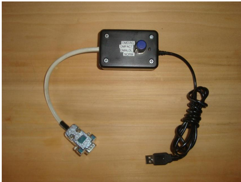
Figure 1 – Fiero ALDL Adapter based on the Adafruit Trinket M0 Microcontroller
